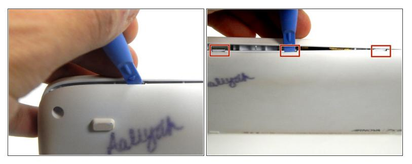
• Place the iFixit opening tool in the notches between the cases and pull the covers apart.
