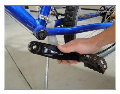
Slide the new crank arm on the the tapered square of the bottom bracket axle.
