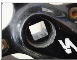
• Clean the bottom bracket axle, crank arm, and sprockets with a rag.
