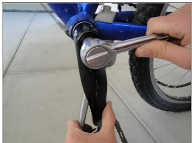
Use a socket wrench to tighten the main bolt.
