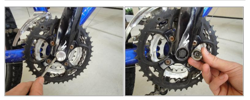
Take cap off the crank arm with flat head screw driver. It should just pop off.
