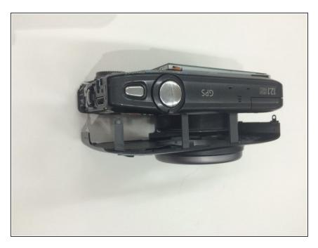
After removing the exterior screws, use your fingers to gently lift off the front face plate.
