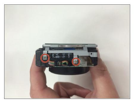
Next, remove the 2 (3 mm) interior screws on the left side of the camera.
