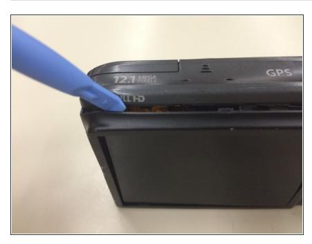
Use your plastic opening tool to gently lift and remove the back face plate.
