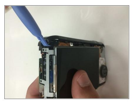
After removing the interior left screws, use a plastic opening tool to gently pull the top face plate off.
