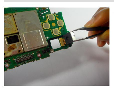
With the camera facing away, pull it from the motherboard until it stands perpendicular to the board.
