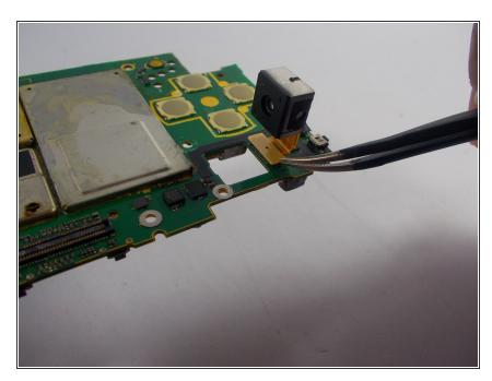
Use tweezers to pull the camera off of the motherboard. Hold on to the plastic connector and apply the force away from the board.
