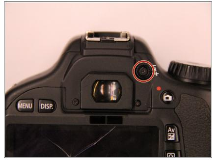
• Remove the screw in the center of the viewfinder focus knob located to the right of the eyepiece.
