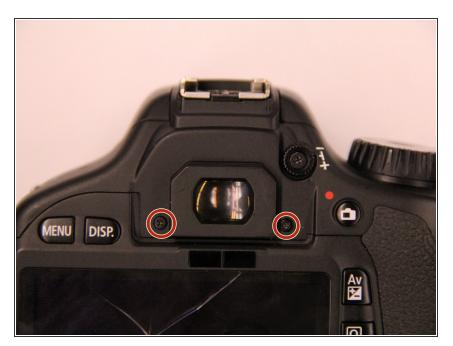
Remove the two screws beneath the eyepiece
