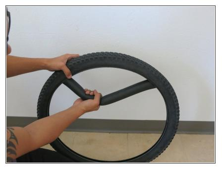
Pull the inner tube away and out of the tire until it is completely detached from the tire.
