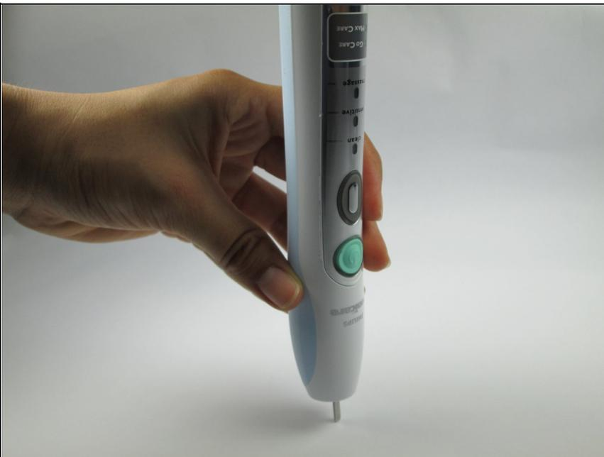
**⚠** The previous version of this step told people to press on the shaft until the electronics were exposed. **DO NOT DO THIS**, it can snap locking tabs off
