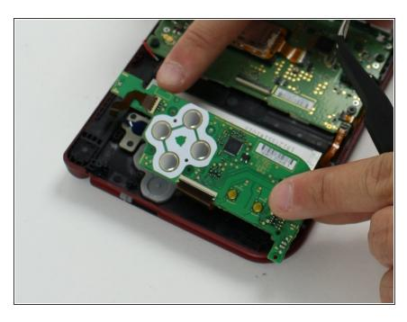
Carefully flip the board over and use tweezers to remove the blue-black ribbon located underneath.
