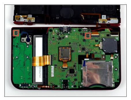
Use non-conductive tweezers to disconnect the two ribbon plugs that connect the L/R/ZL/ZR buttons on the cover to the motherboard, then remove it completely.
