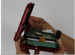
(i) To pry off the cover, carefully lift it up and away from the hinges (in order to clear the headphone port), then pivot it towards the hinges to expose the circuit boards.
