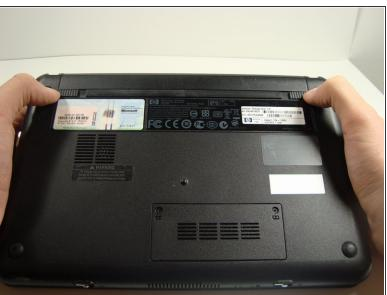
Locate the battery and the battery tabs on the bottom of the Compaq Mini.
