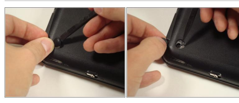
Remove the rubber pads located on the corners of your Compaq Mini.
