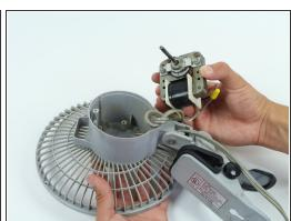
Remove the motor cage from the fan housing.
