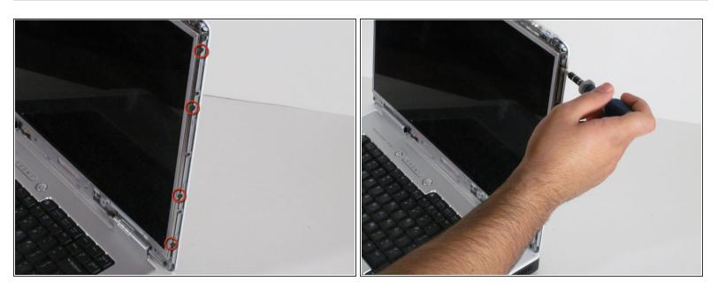
• Remove the 4 screws along the left and right sides of the screen. There are 8 screws in total.
