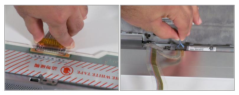
• Remove the two leads from the screen. They will stay connected to the computer.
