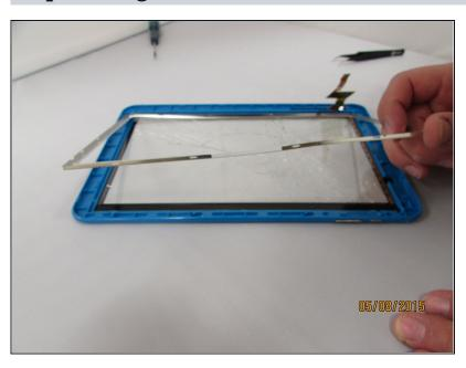
• Simply lift up the loose metal frame and set aside.
