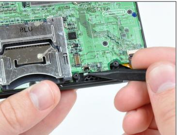
• Use your fingernail or the edge of a plastic opening tool to carefully flip up the touchscreen ribbon cable retaining flap.
