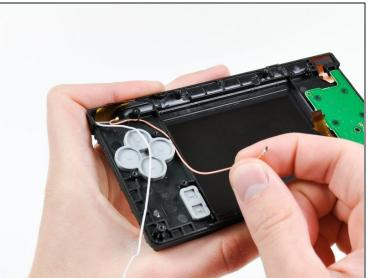
• De-route the Wi-Fi and microphone cables from the slot molded into the bottom front bezel.
