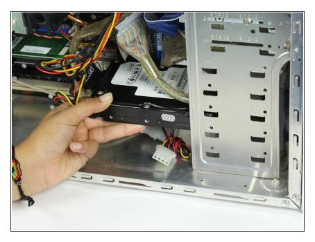
Slide the hard drive out from the metal casing.
