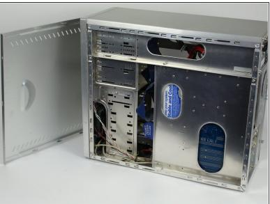
Next, remove the side panel of the computer case to allow access into the computer.
