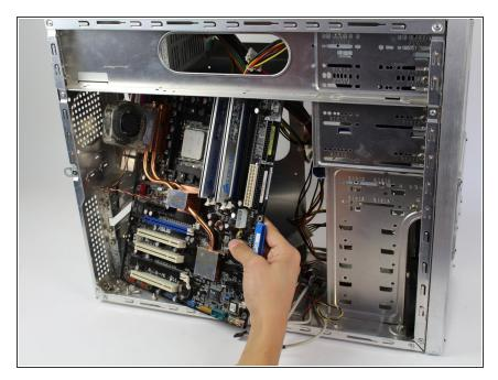
Double check and make sure all wires and screws have been removed, then carefully remove the motherboard from the computer case.
