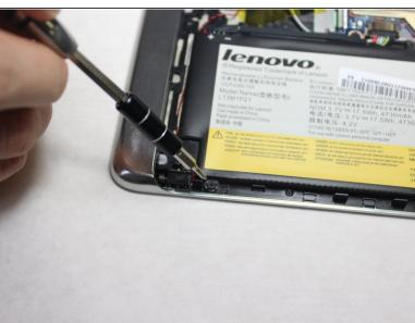
Unscrew the six 3mm screws surrounding the battery dock using a Phillips #0 screwdriver.
