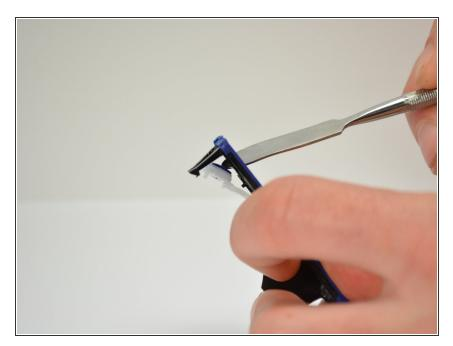
Using the spudger, push the button in and create a small gap between the outside structure and the button.
