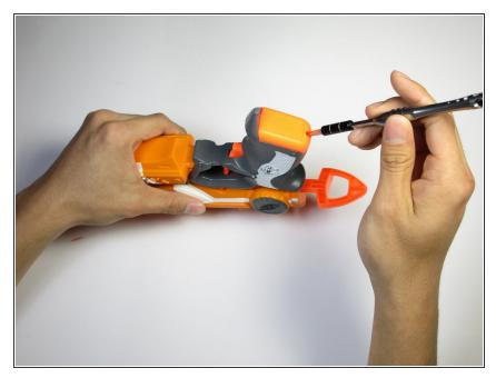
Use a #1 Phillips screwdriver to remove the 10 -mm screw that secures the battery plate, then remove the battery cover using your hands.
