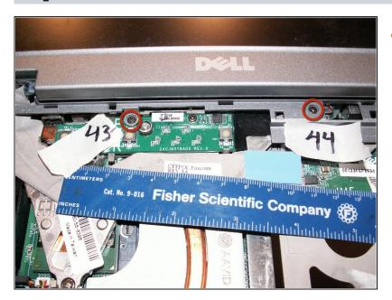
Remove two PH1 5mm bronze screws near the hinge.
