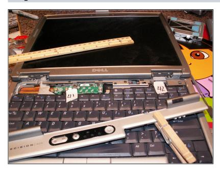
Remove the switch bezel and set it aside.
