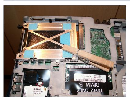
Remove the hard drive cage, shown here with clothespin for emphasis.
