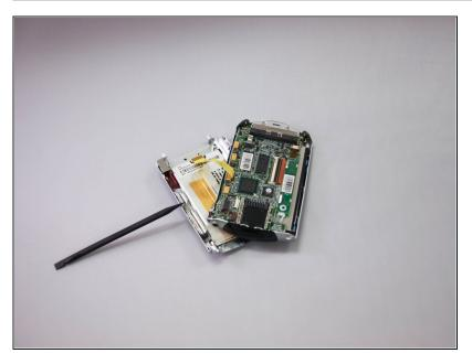
Carefully remove the back cover using a plastic opening tool against the grooves along the sides of the iPAQ.
