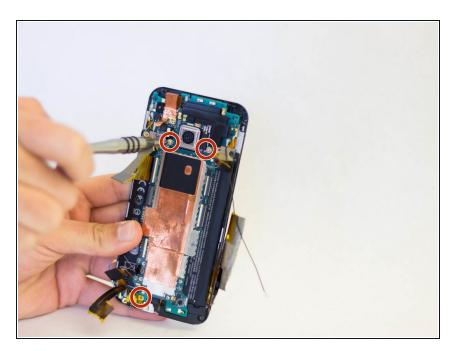
Remove the three 4 mm T5 Torx screws that secure the motherboard.
