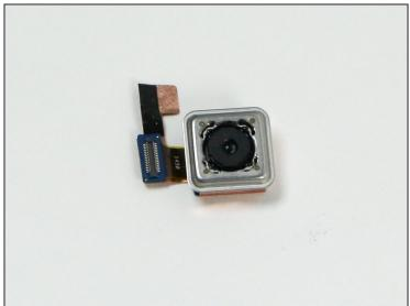
• Flip the daughterboard over and use the tweezers to remove the back camera from the board by applying upward force to the ribbon connection.
