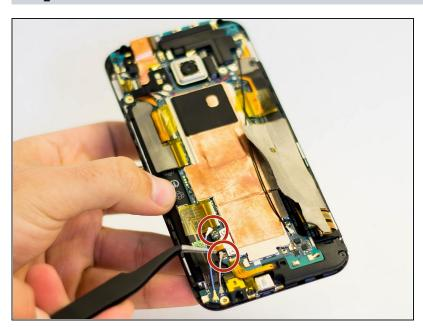
Use a pair of <u>tweezers</u> to get underneath the white and blue cable connectors and gently push them upwards to disconnect them.
