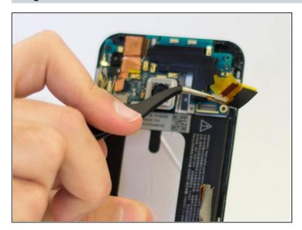
• Using the <u>tweezers</u>, disconnect the ribbon cable.
