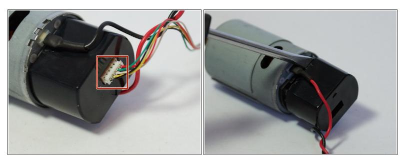
• Remove the white 5-pin adapter from the end of the optical encoder.
