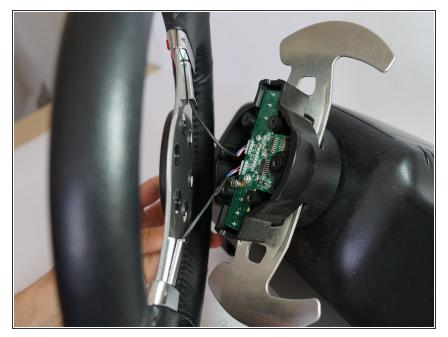
• Carefully lift the wheel off of the hub, exposing the 2 shifter paddle wires and PCB board.
