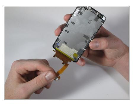
With the front assembly in hand, gently lift back the flat orange wire from the silver backing. The speaker is attached to the silver plate.
