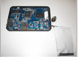
Once you have the back cover off you can see that the battery is help in by double sided sticky tape. Gently pull up on the battery and move it to the side.
