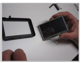
• There are four screws one in each corner. Remove them and gently pull out the LCD Screen keep in mind for the buttons.
