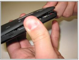
• I used a pair of fingernale clippers to gently pry open the case at the MicroSD card slot. A slight twisting action will pop it off. Just be sure not to go to far in and damage the unit.
