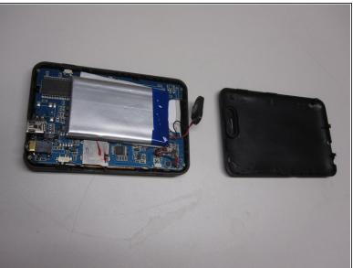
• Be careful when opening the unit. The speaker is attached to the back cover and the wires are fragile. The speaker is held in by some double sided sticky tape. Just use your fingernale and pull up on the edge. DO NOT PULL ON THE WIRES...
