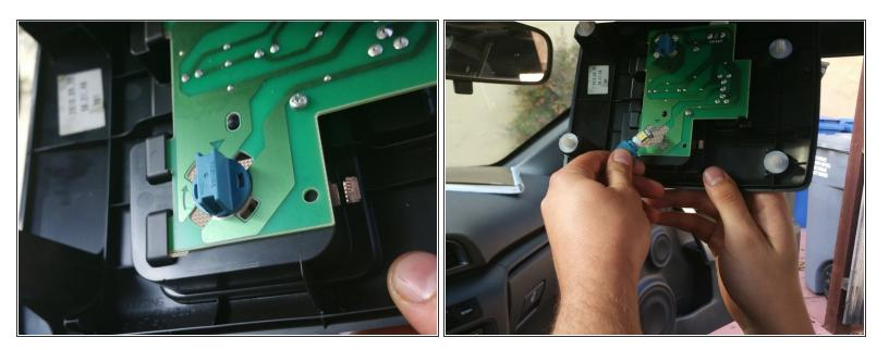
Turn blue knobs counter clockwise and pull to remove bulb housing.
