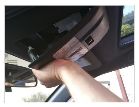
Remove the plastic covering of the lights by pulling it down quickly from the windshield side.
