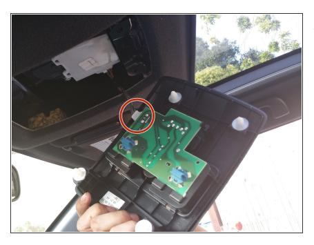
Disconnect the plastic header from system by pressing inward on the side tabs.
