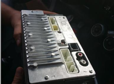
• Remove each bundle of wires that is connected to the back of the head unit.
