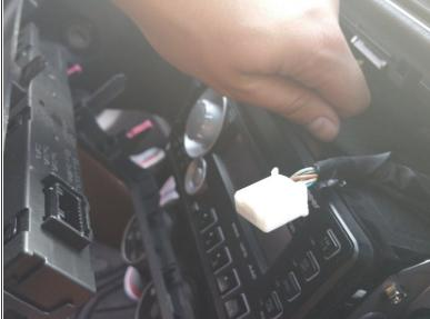
Remove the wire header connected to the panel by pressing inward on the tabs.
