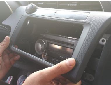
Remove the dashboard panel around the radio head by pulling on the bottom of the unit.
