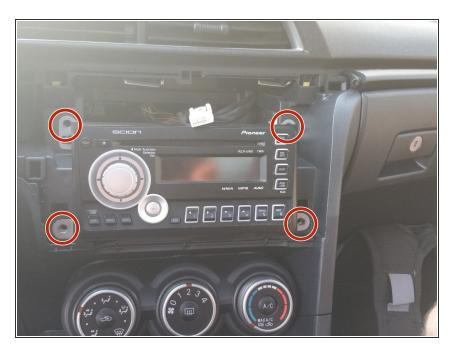
Remove the four #2 12mm screws securing the head unit in the housing
