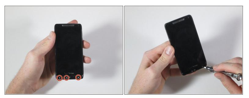
• Remove the three T4 Torx screws. There are three at the bottom of the device.
