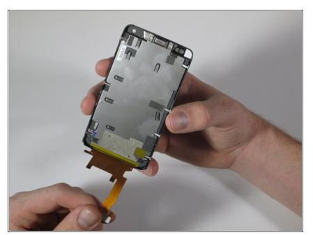
Holding the front assembly, carefully peel back the flat orange wire that is attached to the display from the silver backing. The silver backing is the plating where the speaker is located."
