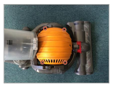
Using a Torx screwdriver, remove the four screws that hold both sides of the ball together.
