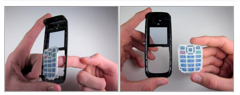
Push on the keypad from the exterior of the phone's front cover to separate the keypad from the phone.
