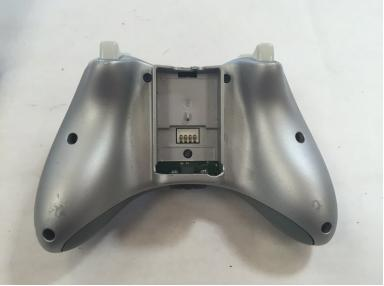
Close controller and replace the screws with the TP Torx T8 Screwdriver.
