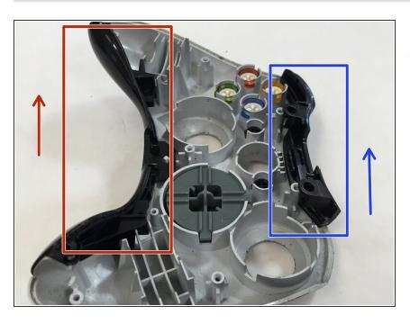
To remove bumper housing and bottom piece, pull away from the shell (along the axis of the screwposts).
