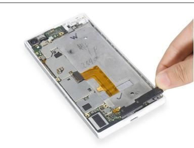
Twist off screws and remove bottom securing bracket.
