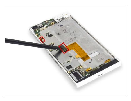
Release power flex connector and LCD screen connector.
