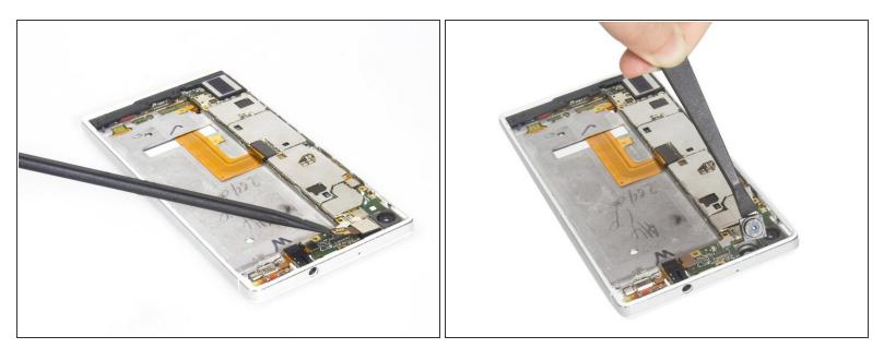
Release connector and remove front facing camera.
