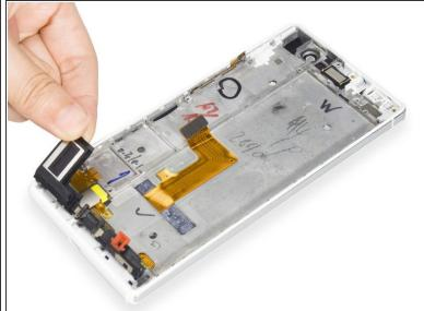
Remove loudspeaker assembly.
