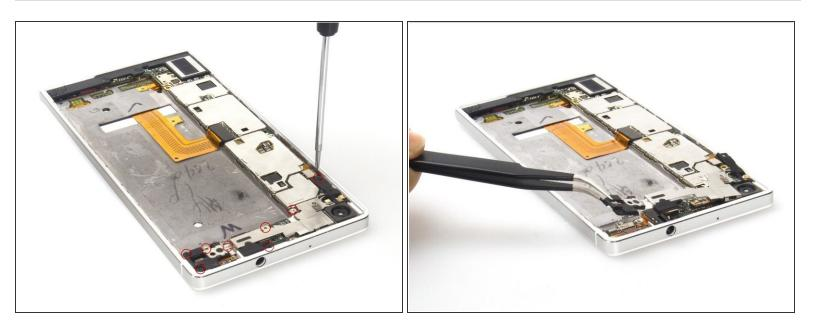
Twist off the screws and remove the top securing bracket.
