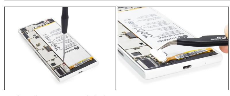
Remove battery connector securing bracket.
