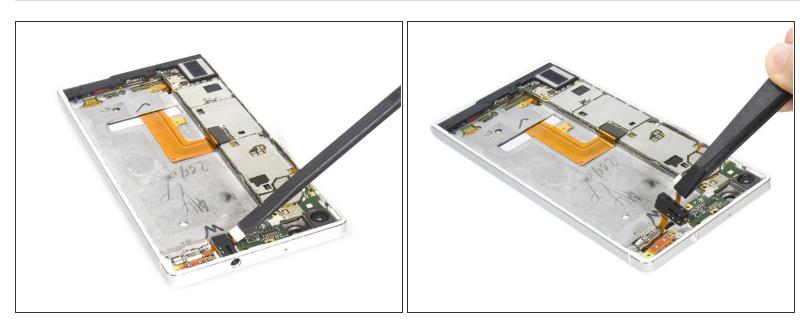
Release the connector and pry to remove headphone jack assembly.
