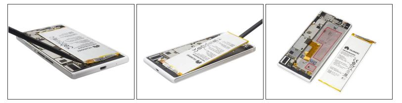
Remove battery. Attention: Be careful with the adhesive and the flex under the battery.
