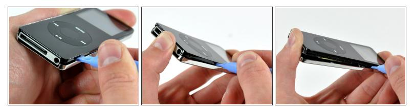
Repeat the same procedure listed in the previous step to free the five clips along the headphone jack side of the iPod.
