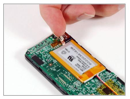
Peel up the ground strap connecting the battery to the logic board.
