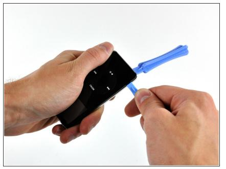
Insert a small iPod opening tool into the seam on the Hold button side of the iPod, with the edge of the tool pointing toward the rear panel.
