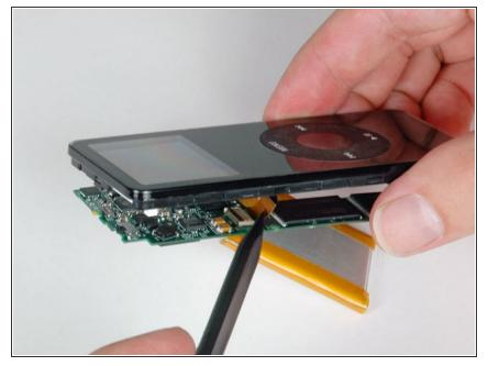
• Use a spudger to slide the display ribbon out of its connector.
