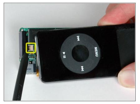
Use a spudger to flip up the black plastic tab holding the orange click wheel ribbon in place. The black tab will rotate up 90 degrees, releasing the ribbon cable.
