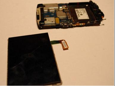
• To remove the screen gently pry up this ribbon cable with a pry tool.
