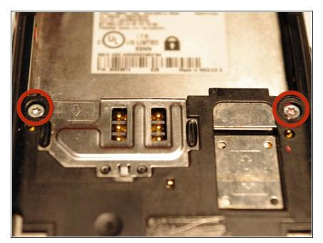
Remove the two hex screws as shown by the SIM card slot.
