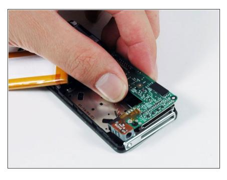
Gently lift up on the dock connector end of the logic board to ensure the logic board is free.
