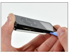
Repeat the same procedure listed in the previous step to free the five clips along the headphone jack side of the iPod.
