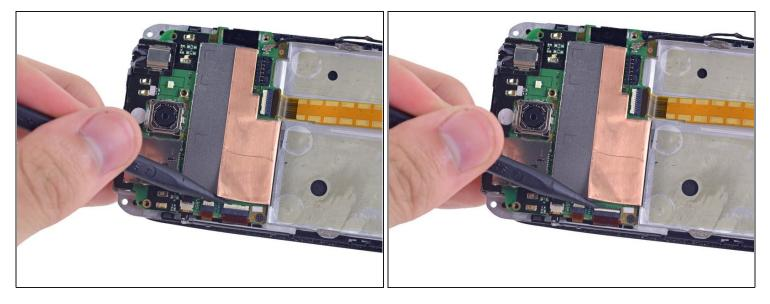
Use the pointed end of a spudger to lift the white tab on the largest ZIF connector opposite the USB connector.
