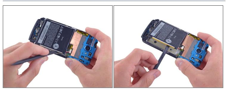
• Switching to the flat end of the spudger, work your way underneath the battery and peel it away from the adhesive.
