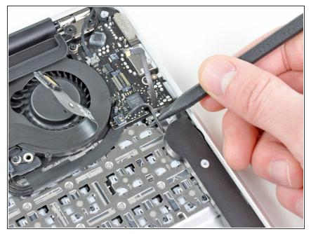
• Use the tip of a spudger to de-route the left speaker cable from the notch cut into the edge of the I/O board.
