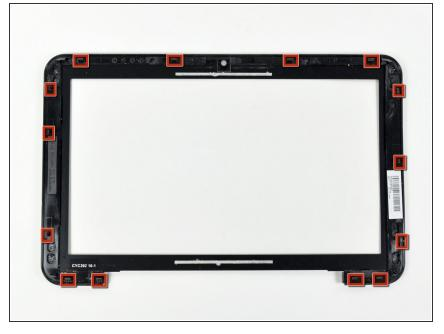
In the following steps you will pry the front display bezel off the rear section of the display. The locations of the retaining clips are highlighted in red.
