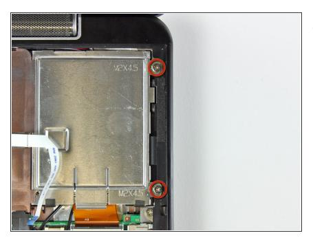
Remove the two 4.5 mm Phillips screws securing the hard drive to the lower case.
