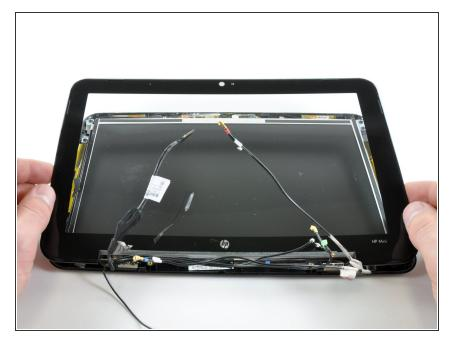
Remove the front display bezel from the rest of the display assembly.
