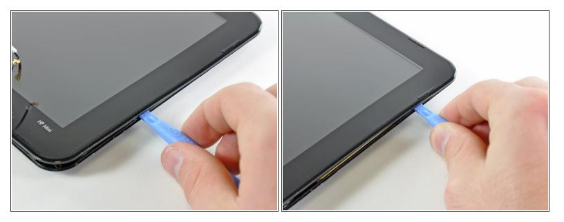
Continue prying to release the clips attaching the front display bezel to the right side of the display's rear section.
