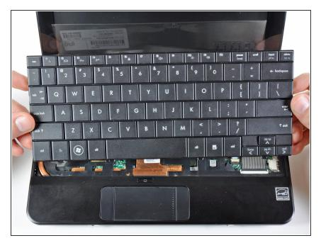
Lift the keyboard out of the upper case, minding the cable that is still connecting it to the motherboard.
