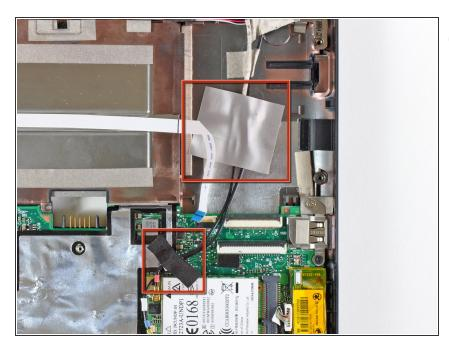
ilf present, remove the pieces of tape securing the Wi-Fi antenna cables to the upper case.
