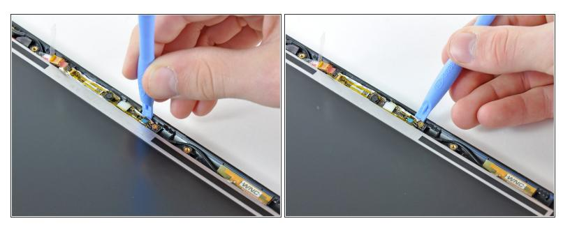
Use the edge of a plastic opening tool to pry the right side of the camera board away from the display assembly.
