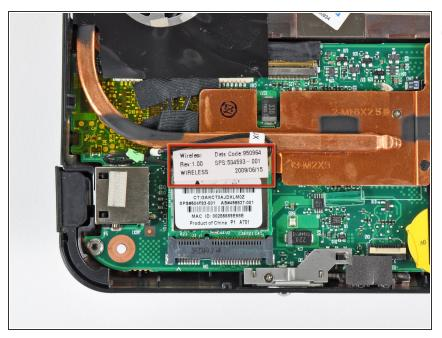
i If present, peel the sticker up off the top of the Wi-Fi board to reveal the Wi-Fi antenna connectors.
