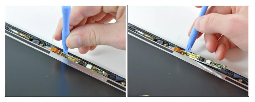
Pry the left side of the camera board away from the display assembly.
