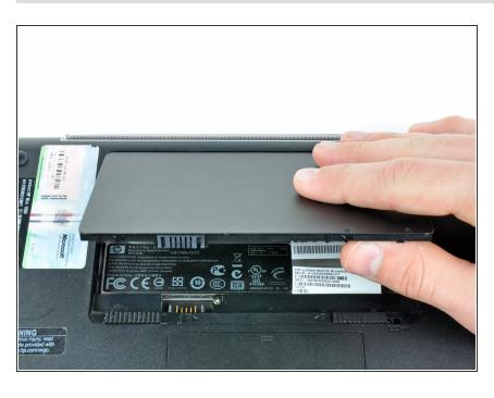
Lift the battery out of the Mini 1000 from the edge closest to the release latches.
