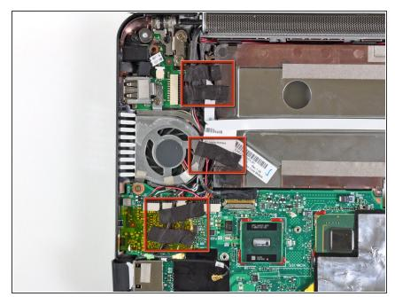
if present, remove the several pieces of black cloth tape securing the cables to the upper case near the fan.
