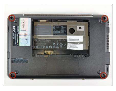
Remove the four 7 mm Phillips screws that secure the upper case to the lower case.
