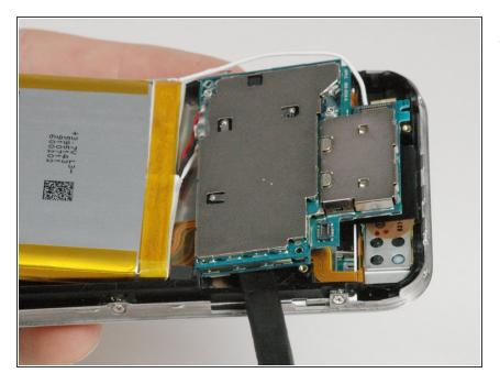
Slide a spudger beneath the logic board on the side opposite the battery connector and pry up slightly. Don't lift up too far, because there are still four attached connectors on the bottom of the logic board.
