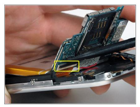
Slide a spudger beneath the black locking bar and pry up to rotate the bar 90 degrees (the bar is already rotated in the picture).
