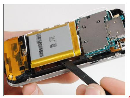
• Working from the edge opposite the battery connectors, insert a spudger between the battery and the plastic frame and pry up on the battery. It is attached to the casing with an adhesive, but should slowly come free.
