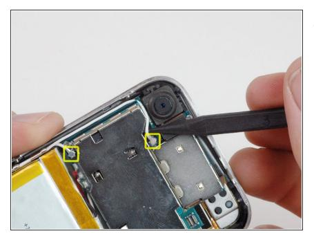
• Use a spudger to disconnect the two antenna cables from the communications board. Apple used a small dab of glue on these connections, which may make removing the antenna connections harder.
