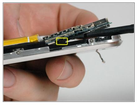
Go to the other side of the logic board and use a spudger to disconnect the touch sensor cable on the under side of the logic board.
