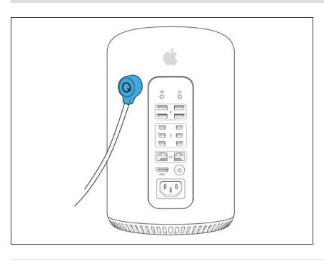
Return the enclosure and slide the latch back to the left. Install cable lock into the exposed hole.
