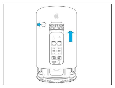
Remove the enclosure by sliding the latch to the right and lifting the enclosure up.
