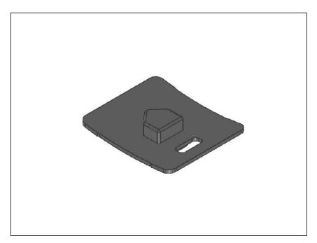
Remove the original latch, install the replacement latch with Kensington lock hole, and restore the retainer plate and six screws.
