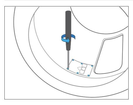
Using a <u>T5 screwdriver</u>, remove the six screws retaining the latch on the inside of the enclosure and lift out the retainer plate.
