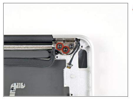
Remove the two 4.9 mm T8 Torx screw securing the antenna cable retainer on the left display hinge to the upper case.
