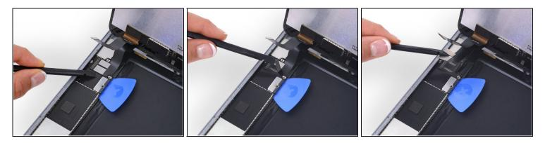
• Disconnect the two remaining digitizer cables underneath the display data cable.
