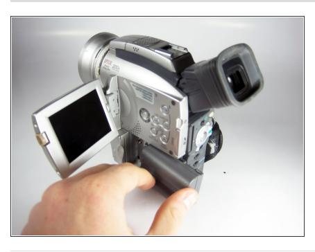
While holding the battery release button to the side, slide the battery towards you, past the release button.
