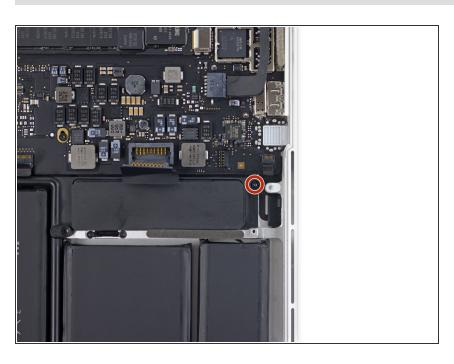
Remove the single 3.7 mm T5 Torx screw securing the battery board to the upper case. To reassemble your device, follow these instructions in reverse order.
