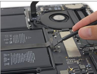
Use the flat end of a spudger to pop the trackpad connector straight up off its socket on the logic board.
