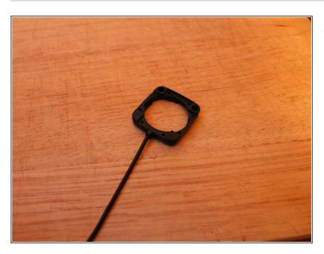
Apply some glue to the mount and re-attach the cap to the mount.
