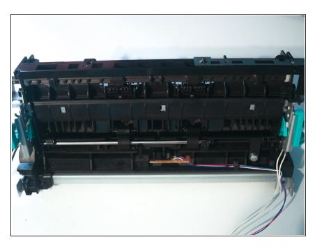
The fuser can now be removed from the printer.
