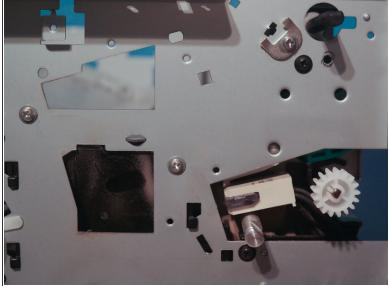
Remove one gear on the output shaft of the fuser.
