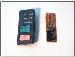
The control panel and its circuit board can easily be removed with a metal spudger.
