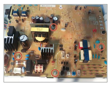
Remove 4 screws on the control board to remove it from the metal plate.
