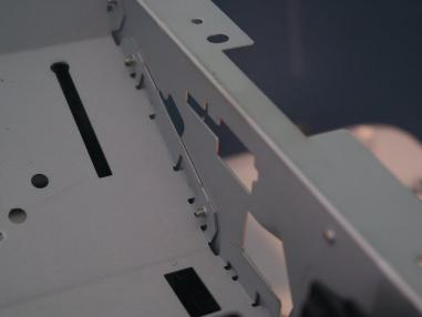
The cable clip for the laser assembly cable can be removed from the chassis.
