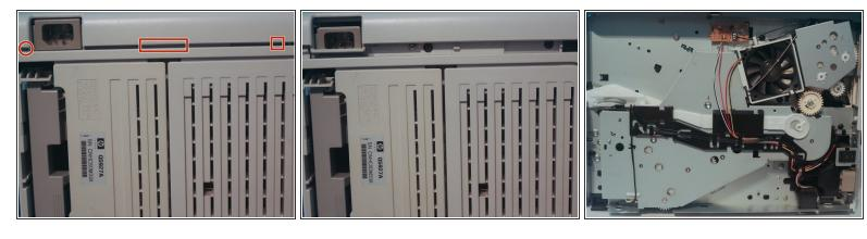
• Removing the right cover is as easy as disengaging 3 tabs with the printer turned on its side.
