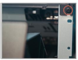
Remove 2 screws on the back of the printer, one on the left side, and one on the front.
