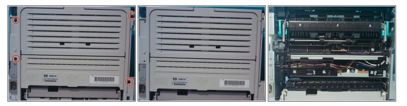
• The back cover can be removed by removing 4 screws on the back of the printer.
