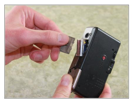
Remove the battery from the camera by pulling the battery door outward.
