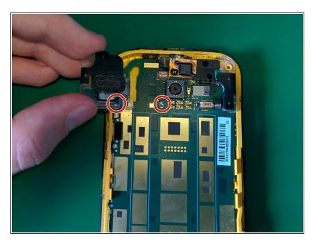
Remove two black Phillips head screws and remove the back speaker assembly.
