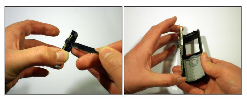
• The microphone is carefully lifted from its bracket, and the motherboard is carefully removed.
