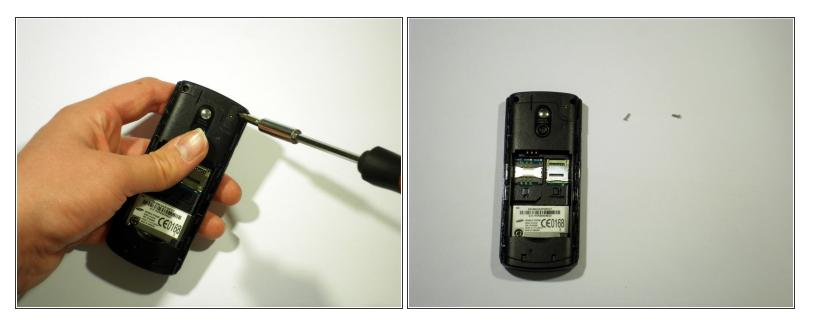
• Next, using a Philips screwdriver, remove the five screws from the back of the device.
