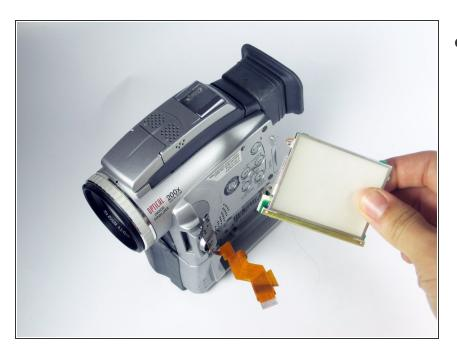
Replace the broken LCD with a new one.
