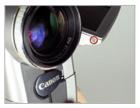
Remove the two 4mm #00 Phillips screws on the inside edge of the LCD casing. After removing the first screw you will have to rotate the screen 180 degrees to remove the second screw.
