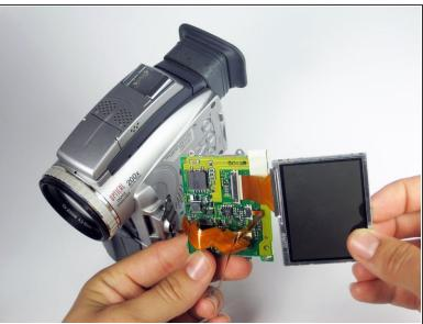
Remove the lower casing by pushing up on the glass screen with your thumb.
