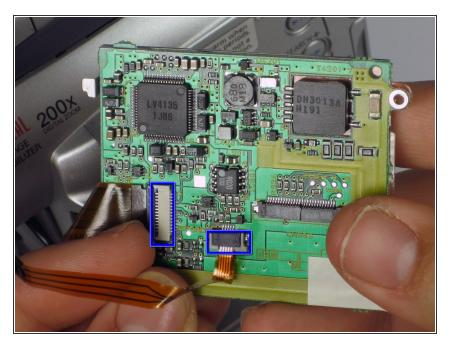
Remove the LCD by disconnecting the remaining two ribbon wires by lifting up the cream-colored gate and sliding the ribbon out of the black gate.
