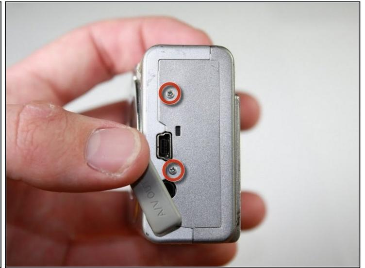
① Position the camera so that the rubber "AV Out Digital" tab is facing upward.
